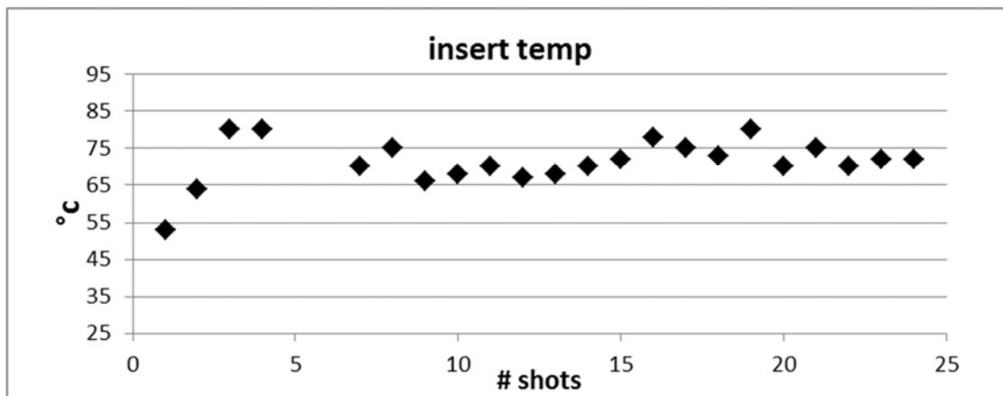
Figure 5: Shot to shot variation of insert's surface temperature
