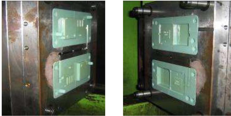
Figure 3: Mold base and PIMT inserts: Left: moving plate (core), Right: stationary plate (cavity).
