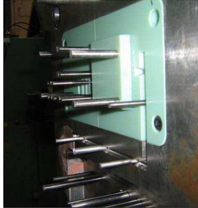
**Figure 4: Ejector pins through PIMT insert**
