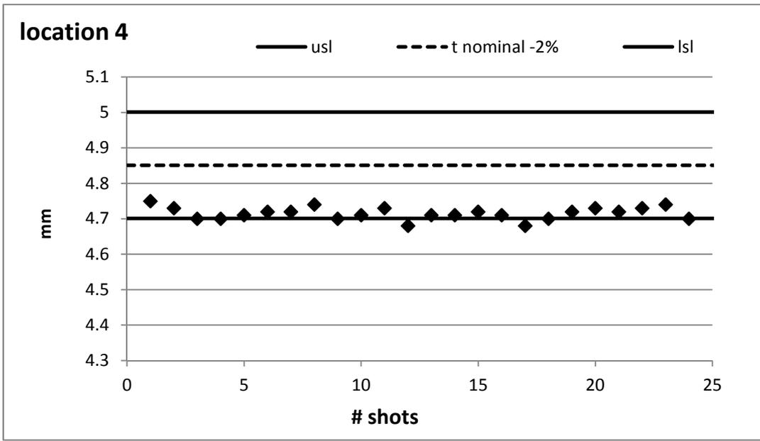
Figure 10: Parts dimension variation in location 4 – thick wall thickness
