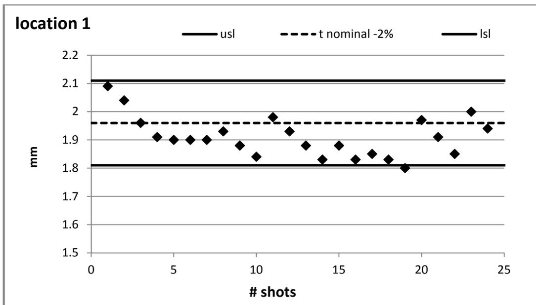
Figure 7: Parts dimension variation in location 1 – lid thickness
