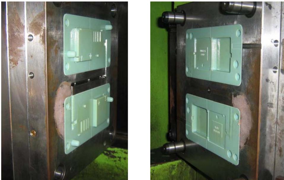
**Figure 2: Mold base and PIMT inserts: Left: moving plate (Cavity), Right: stationary plate (Core)**
