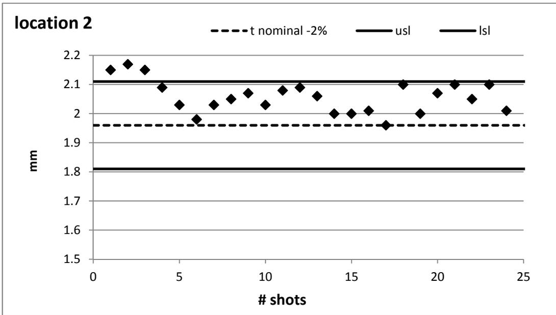
Figure 8: Parts dimension variation in location 2 – box’s wall thickness
