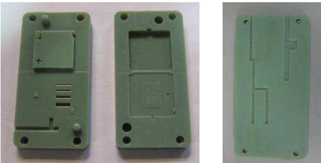
Figure 2 – IM "generic" part PIMT. Left: core and cavity, Right: core opposite side (venting details)
