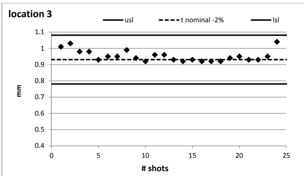
Figure 9: Parts dimension variation in location 3 – thin wall thickness
