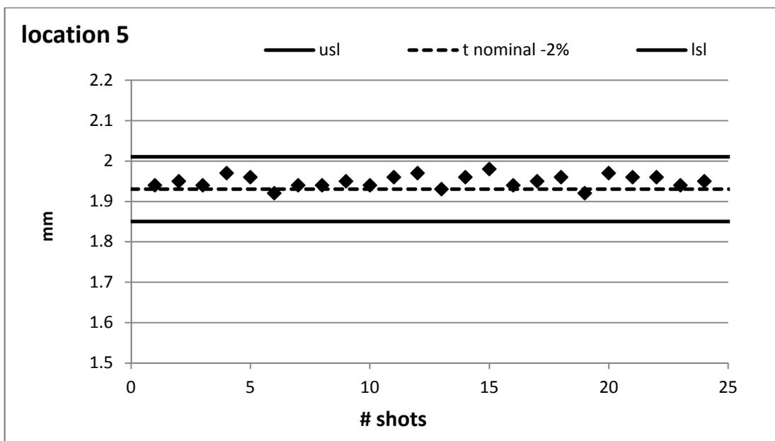
Figure 11: Parts dimension variation in location 5 – boss's diameter
