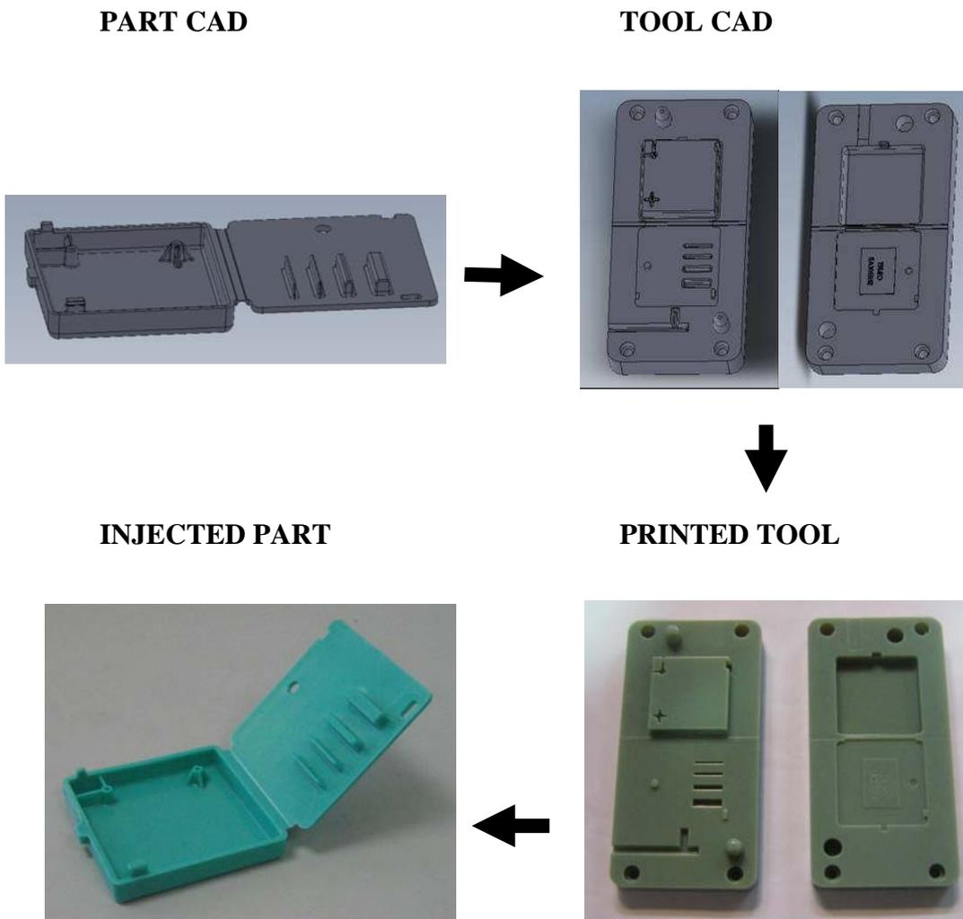
**Figure 1: From CAD to part in only a few hours!!!**
